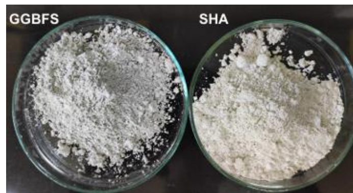
Figure 19. GGBFS after milling and SHA as received
