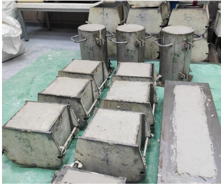
Figure 22. Example of the sealed curing of the concrete samples
