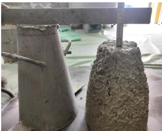
Figure 69. Slump test of the reference mix
