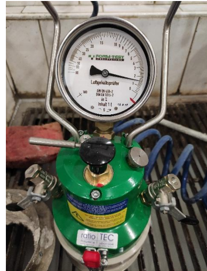
Figure 27. Determination of the air content of concrete by the pressure method
