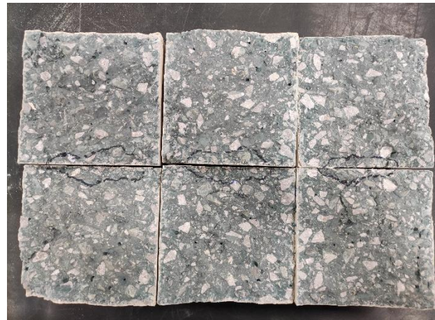
Figure 33. Example of the samples after exposure to water under pressure
