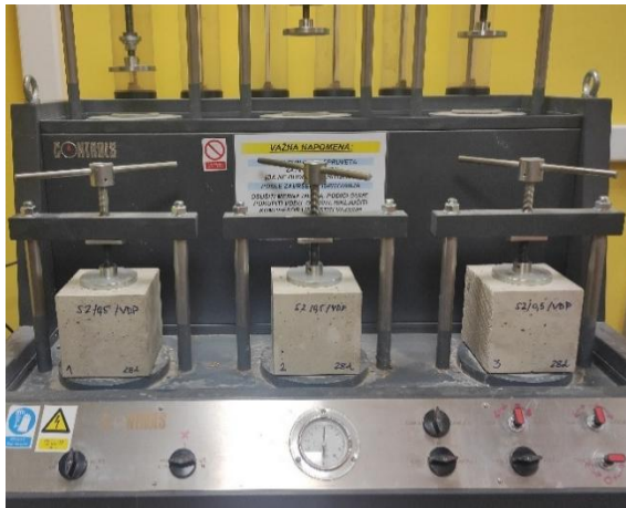
Figure 32. Set up for testing the water permeability under pressure of the concrete samples
