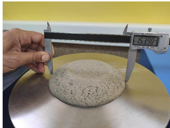
Figure 24. Measurement of the consistency of mortars by the flow table test
