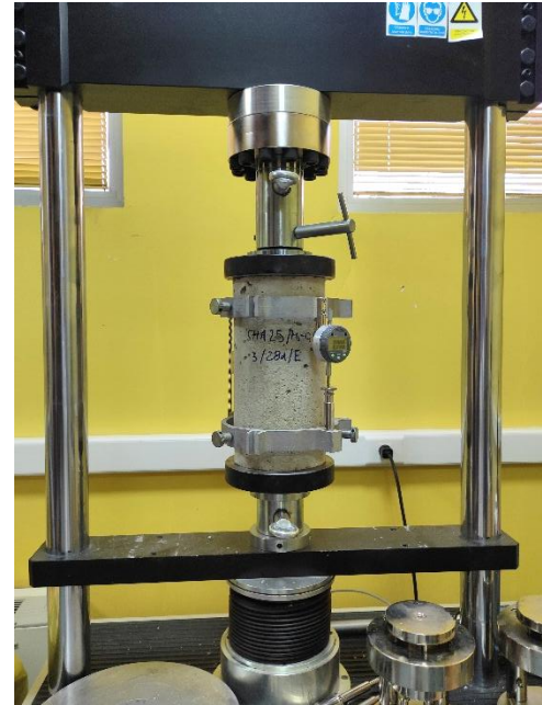
Figure 31. Set up for testing the modulus of elasticity of concrete samples
