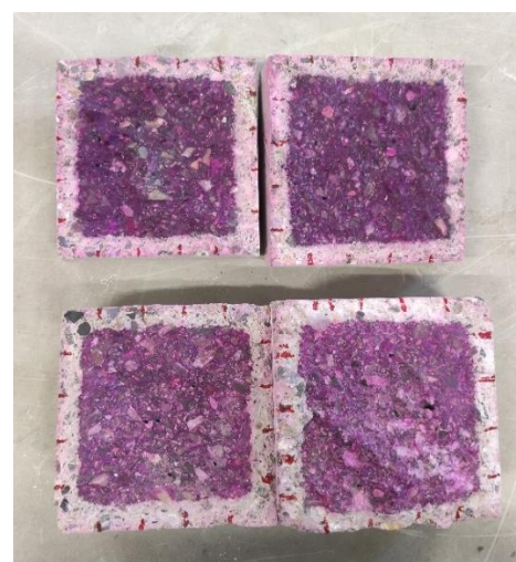
Figure 35. Concrete samples after 28 days of exposure to accelerated carbonation
