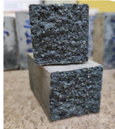
Figure 55. Example of a sample cross-section after testing of the compressive strength
