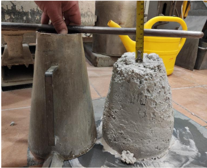
Figure 26. Example of a slump test of concrete
