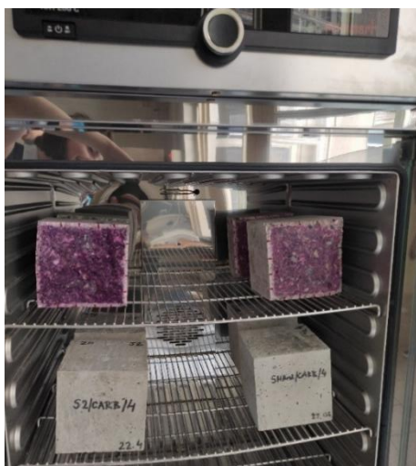
Figure 34. Concrete samples in the carbonation chamber
