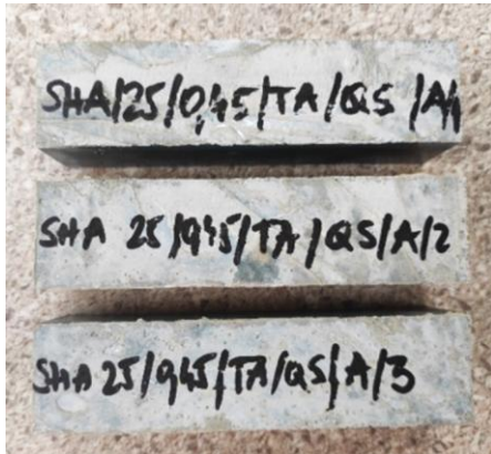
Figure 54. Example of hardened samples before compressive-strength testing
