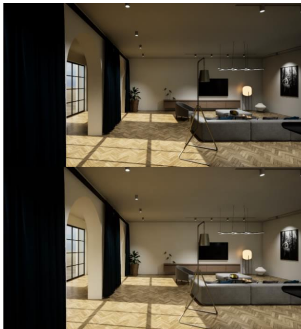
Slika 6. Software ray tracing (gore), Hardware ray tracing (dole)
