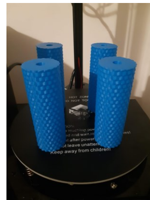
Image 2. Printed rollers on FDM 3D printer
