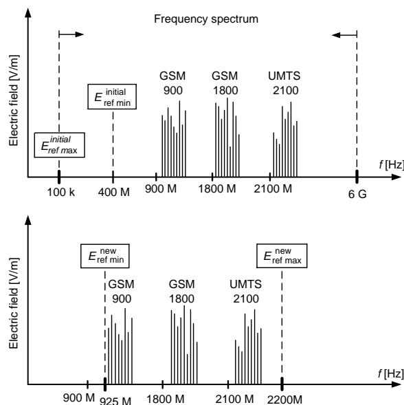
Figure 3: Shrinking of the observed frequency range.
