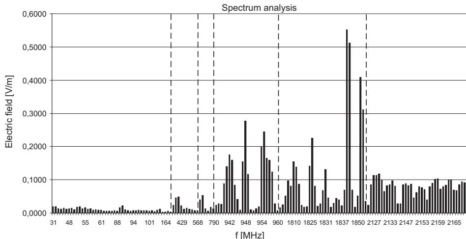
**Fig. 6.** The spectrum of the high-frequency electric field at the measurement location.
